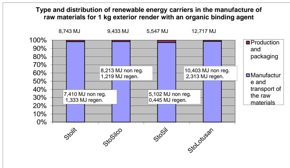
**Illustration 4: Relative primary energy use for production and transport of raw materials, production and packaging of 1 kg of exterior plaster with organic binder.**
