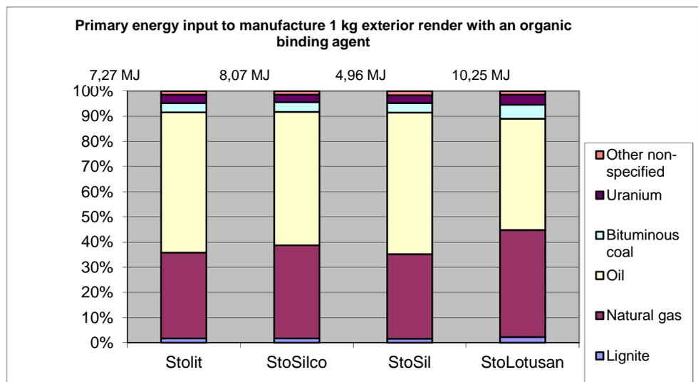
**Illustration 2: Type and distribution of non-renewable energy sources for production of the raw materials for 1 kg of exterior plaster with organic binder.**
