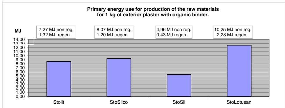
**Illustration 1: Primary energy use for production of the raw materials for 1 kg of exterior plaster with organic binder.**
