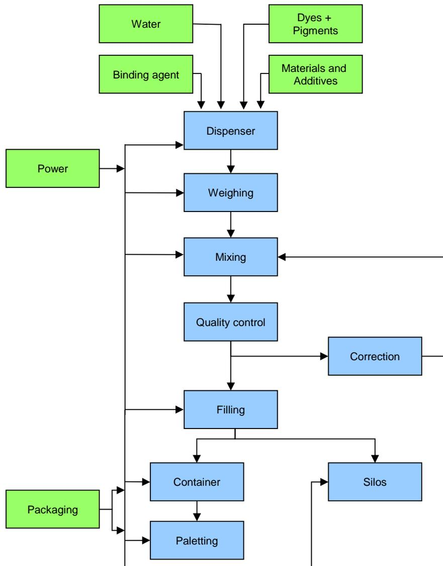
Exterior plasters with organic binders are manufactured in mixing plants in the following work steps:
