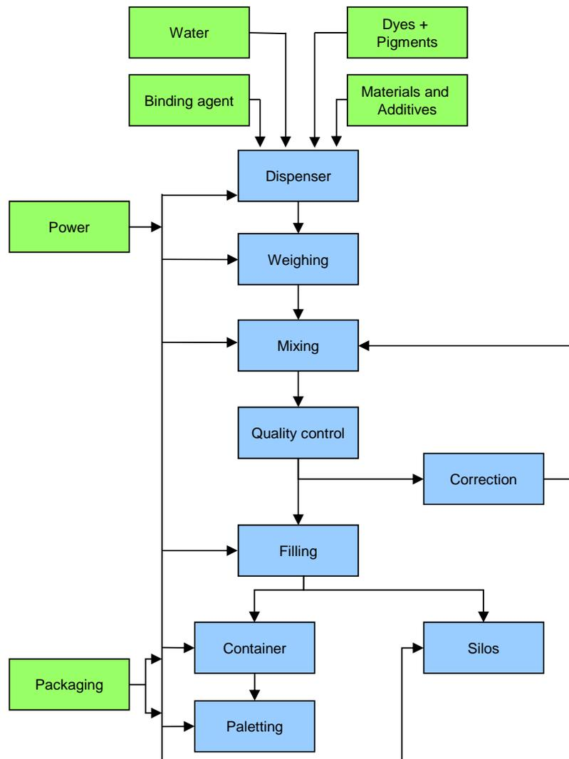
Facade paints and primers are manufactured in mixing plants in the following work steps:
