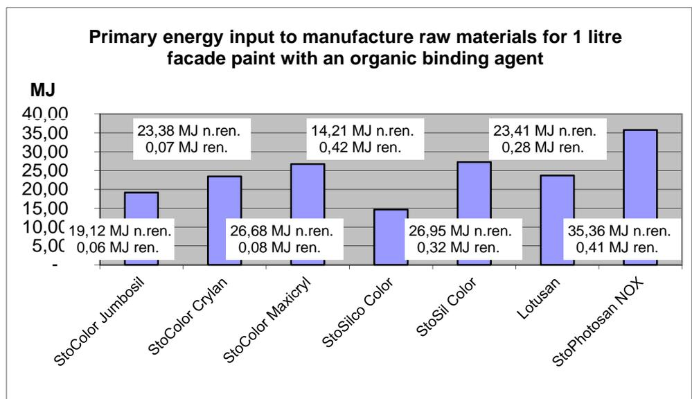
**Illustration 2: Primary energy use for production of the raw materials for 1 litre of facade paint with organic binder**
